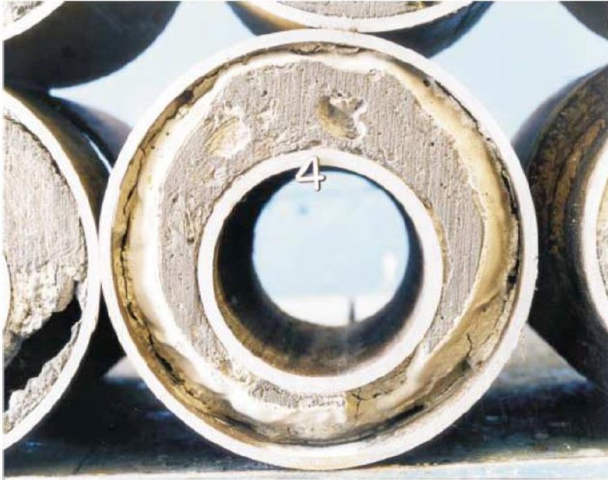
Figure 2.6. Incomplete displacement of drilling mud and the resulting drilling mud channels. Over time, the gels in the drilling mud will shrink, forming fluid migration pathway in the annulus (after Watson 2004).
