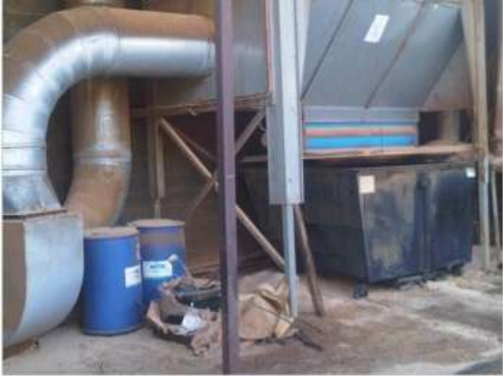
Image 5. Dry shavings handled with exhaust ventilation system to hopper at North Eden Hardwoods
