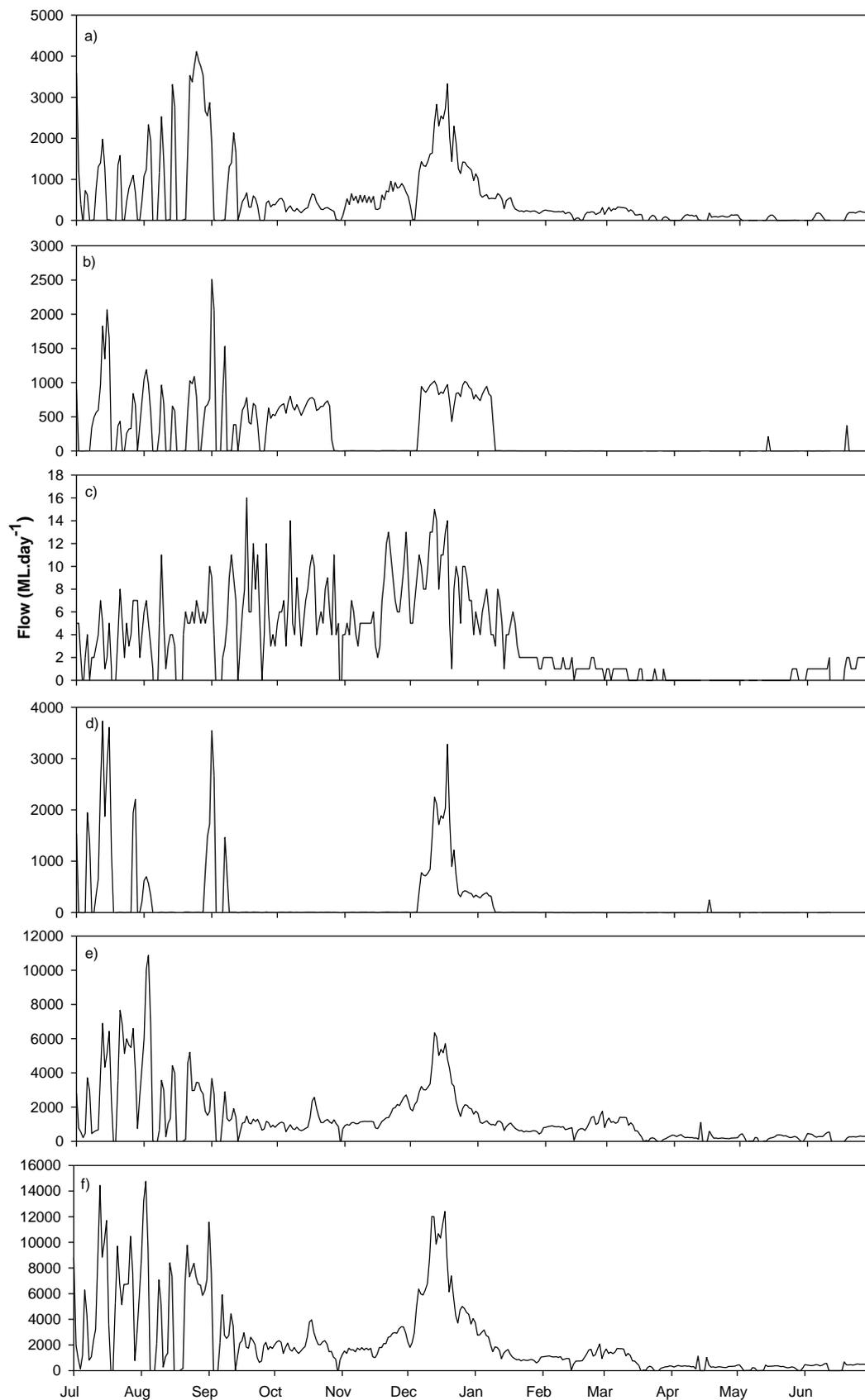
**Figure 3-2. Daily flow discharge by individual barrages (ML.day<sup>-1</sup>) for 2017-18. a) Goolwa barrage, b) Mundoo barrage, c) Boundary Creek barrage, d) Ewe Island barrage, e) Tauwitchere barrage and f) Combined discharge (five barrages). Data source: DEW.**
