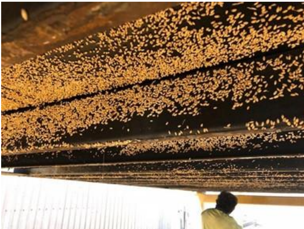
Seed contamination on the underside of a sea container. Image courtesy of the Australian Department of Agriculture, Fisheries and Forestry.
