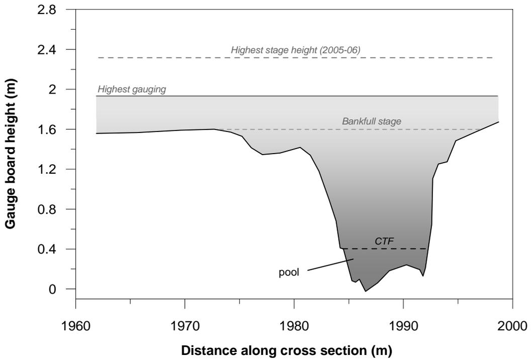
**Figure 3.3** Cross section at GCUS taken during August 2005. CTF = cease-to-flow.
