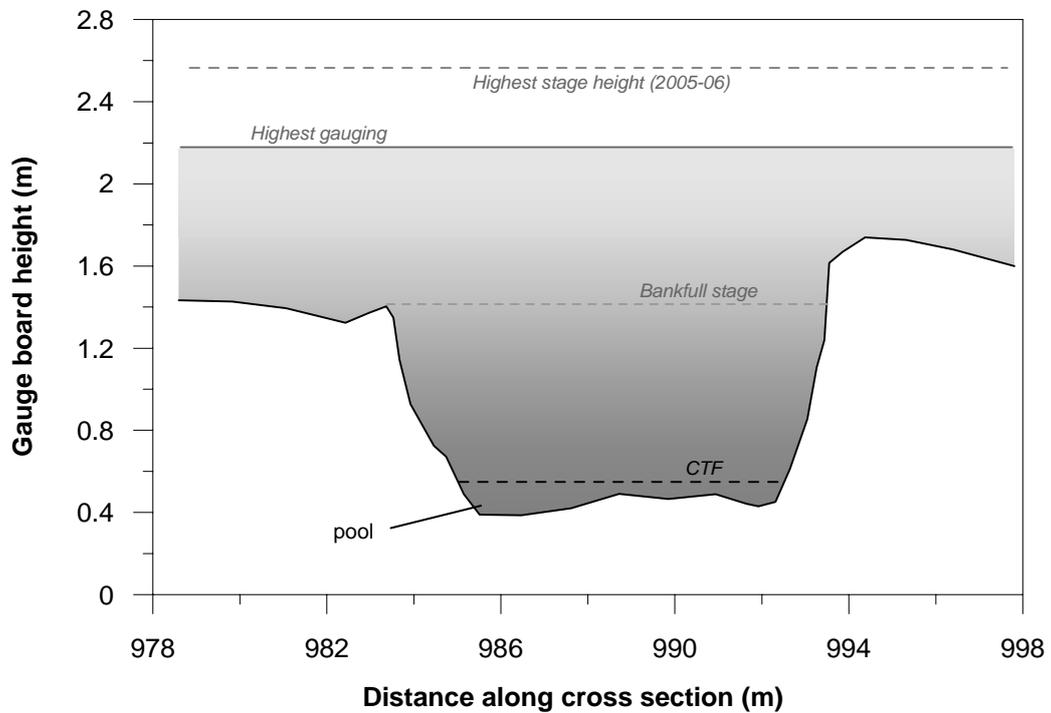
Figure 3.7 Cross section at GCDS taken during September 2005. CTF = cease-to-flow.
