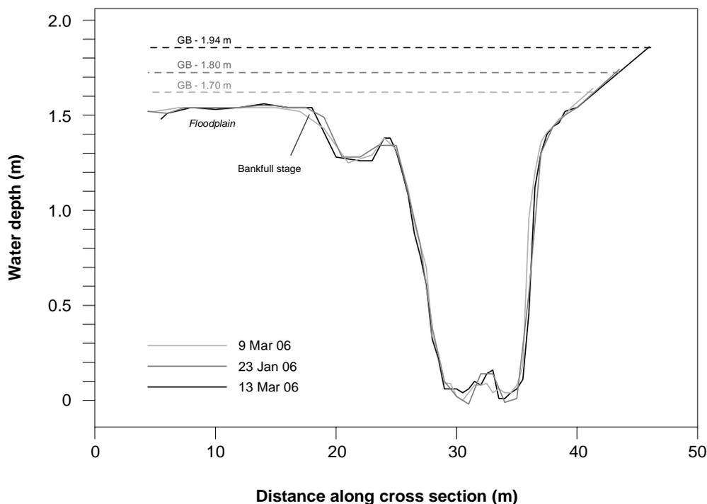
**Figure 3.1** Cross sections at GCUS taken during three overbank flow gaugings during the 2005–06 wet season
