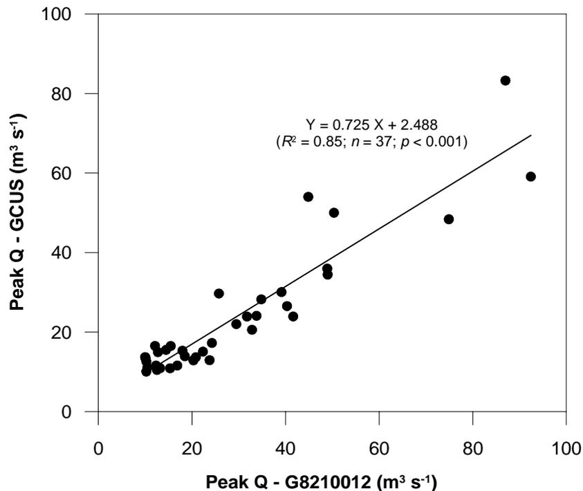
Figure 3.9a Fitted relationship between peak flood discharges observed at GCUS and G8210012
