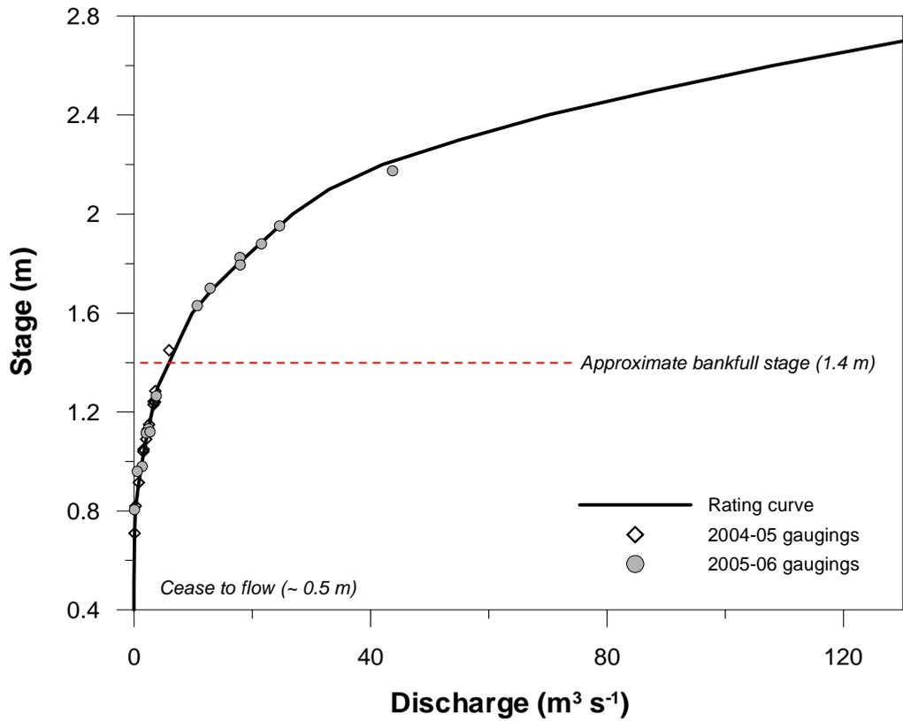
Figure 3.6 Rating curve for GCDS with the gauging points shown
