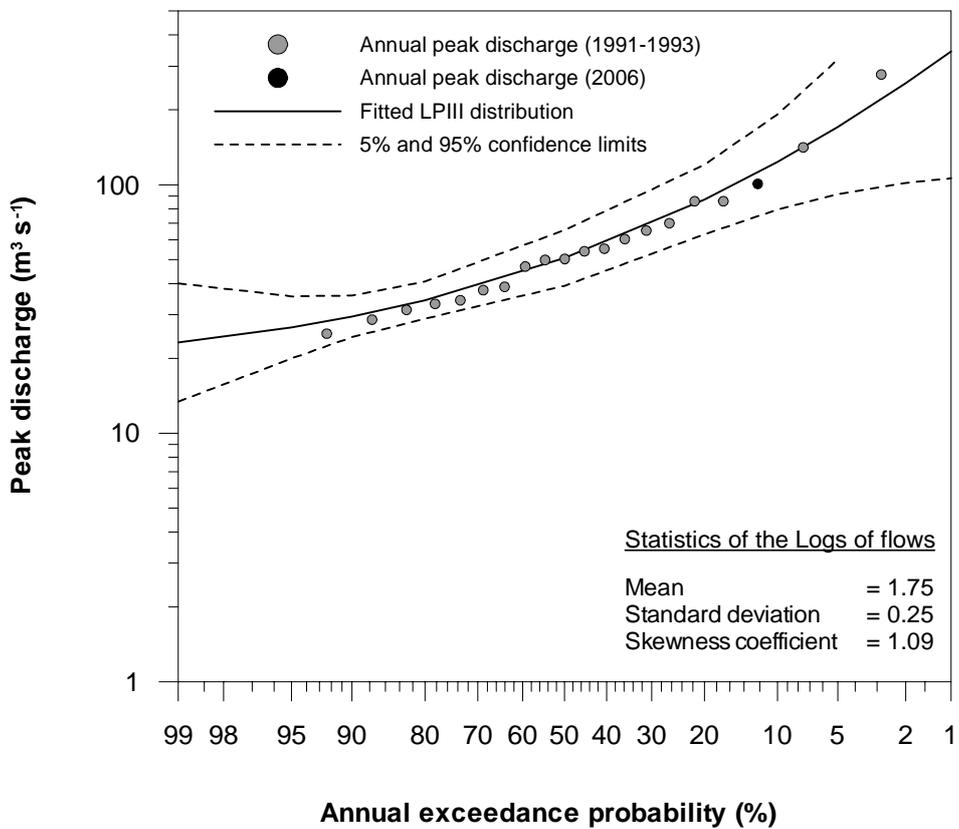
**Figure 3.11** Frequency curve of annual peak discharge at GCDS
