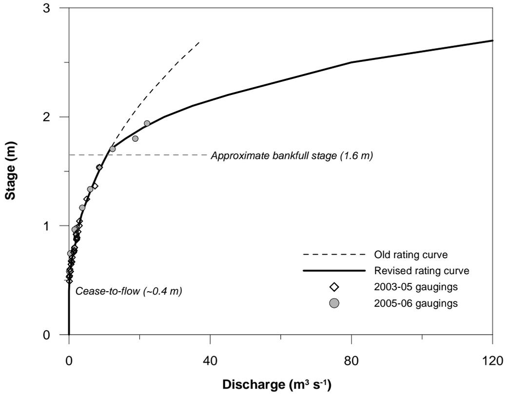
**Figure 3.2** Revised rating curve for GCUS with the gauging points shown. Old rating curve for GCUS is also shown.
