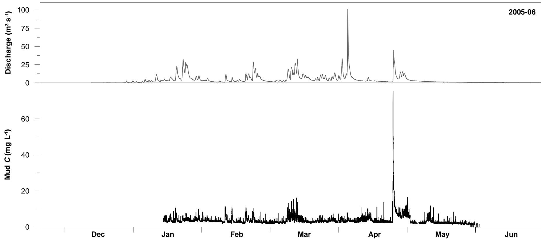
**Figure 4.3b** Continuous mud C data derived from the turbidimeter record for the 2005–06 wet season at GCDS. Discharge data are also shown.
