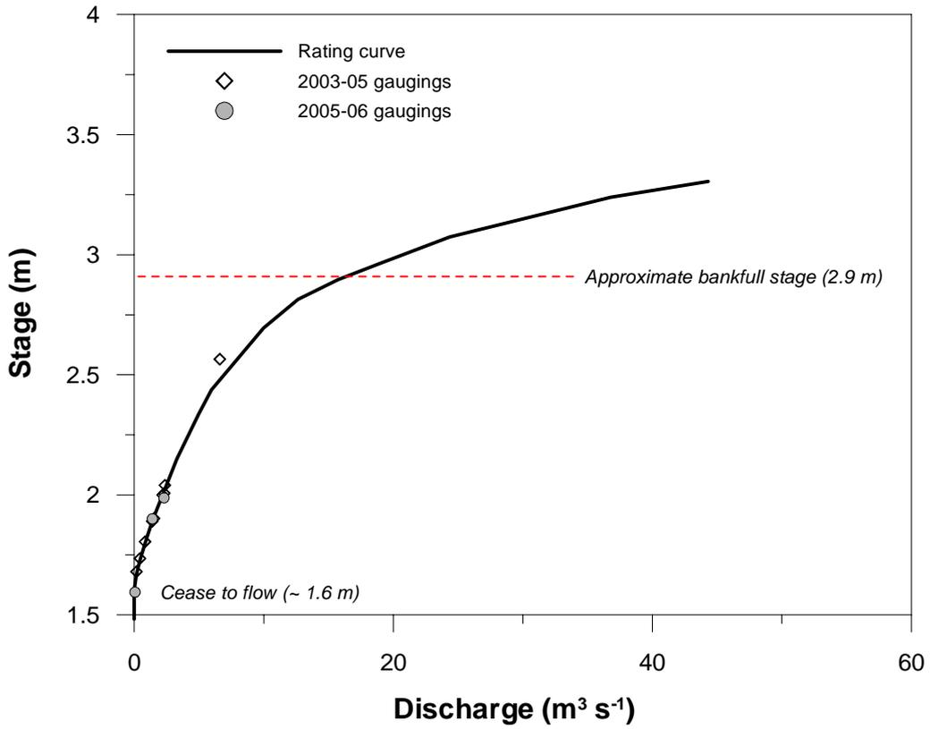
Figure 3.4 Rating curve for G8210012 with the gauging points shown
