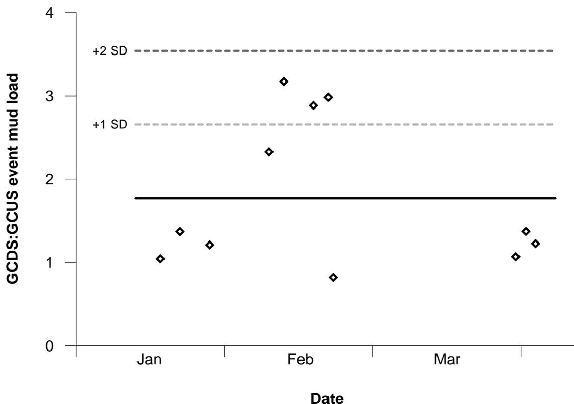
**Figure 4.4** Temporal variation of the ratio of event mud loads measured at GCDS to that at GCUS during 2005–06 (indicated as  $\diamond$ ). The mean ratio and associated standard deviations are also shown.
