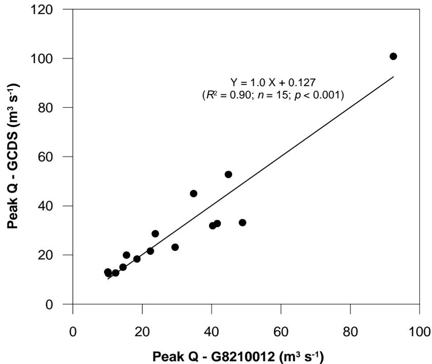
**Figure 3.9b** Fitted relationships between peak flood discharges observed at GCDS and G8210012
