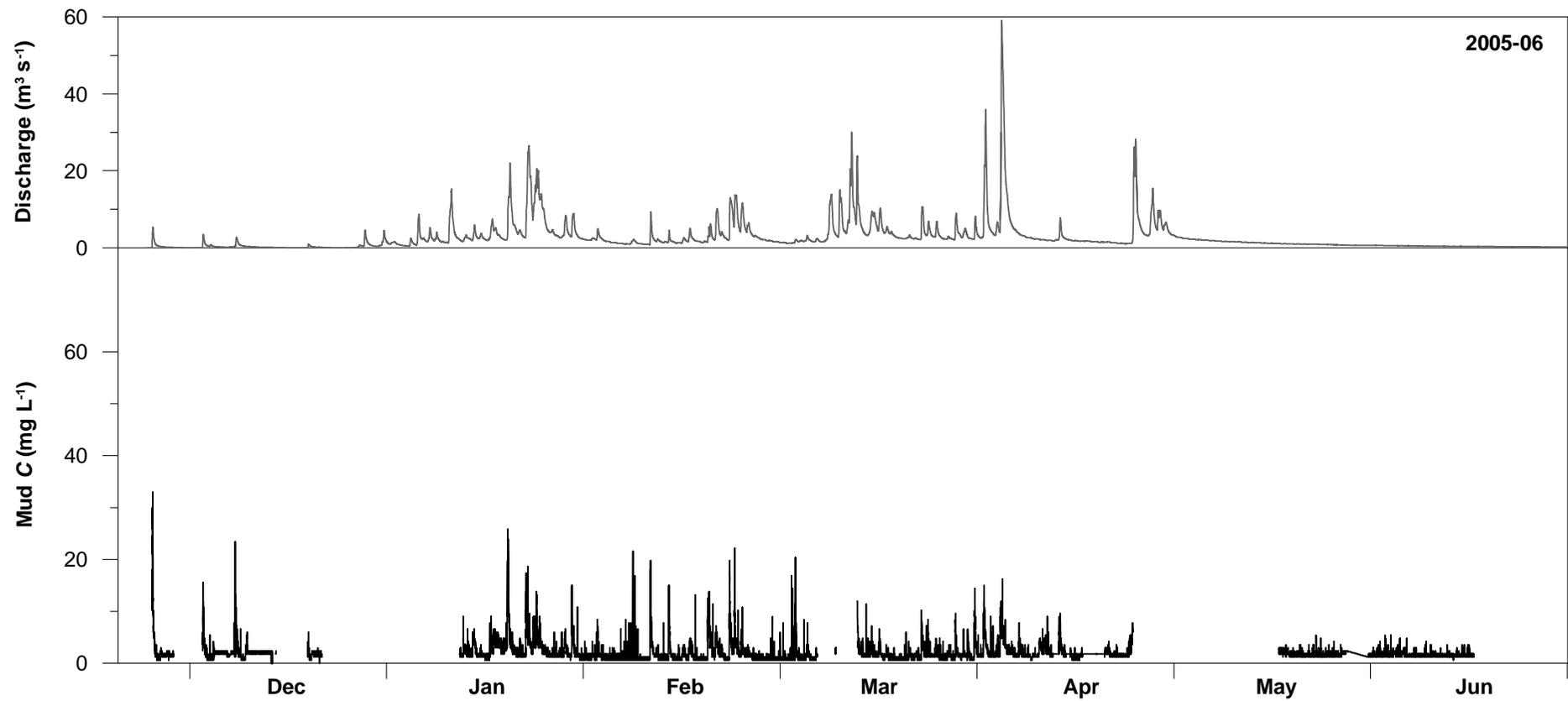
Figure 4.3a Continuous mud C data derived from the turbidimeter record for the 2005–06 wet season at GCUS. Discharge data are also shown.
