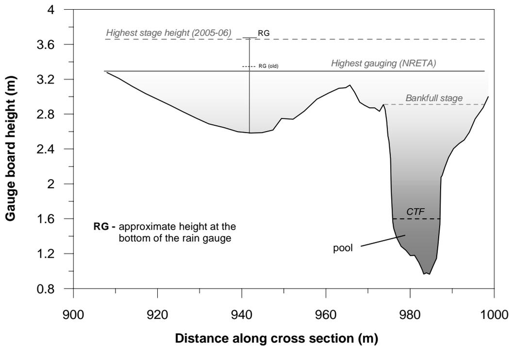
Figure 3.5 Cross section at G8210012 taken during August 2005. CTF = cease-to-flow.
