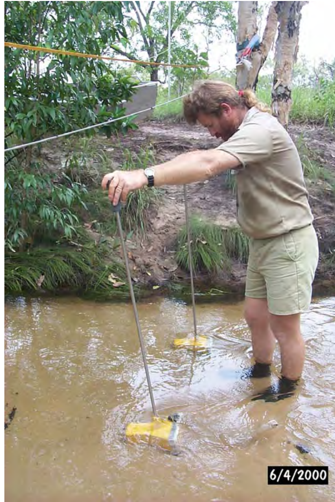
Figure 2 Bedload samples being collected at the Swift Creek site. Where possible two samplers were used to collect samples on each transect, thus reducing collection time.
