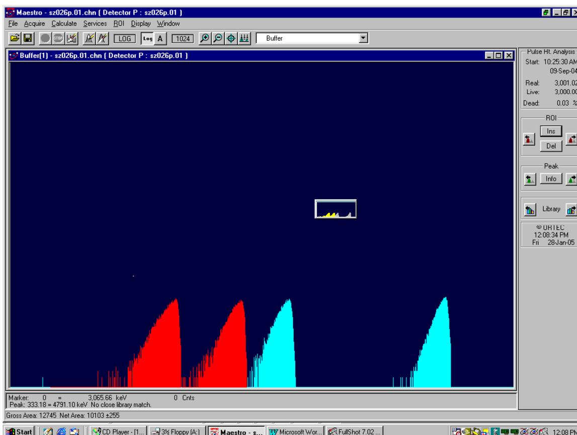
Figure A4.4 A complete set of ROIs for  $^{226}\text{Ra}$  analysis
