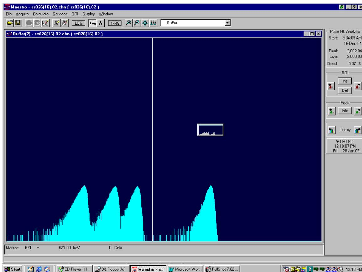
Figure A4.5 Spectrum with poor resolution of peaks
