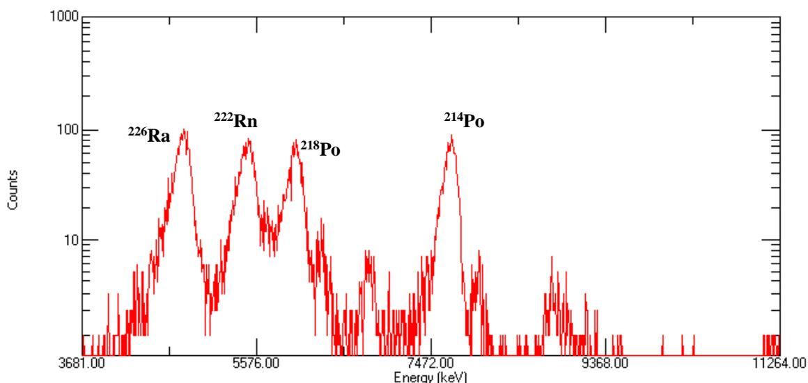
**Figure 2** Very poorly resolved spectrum from Ba interference on disc
