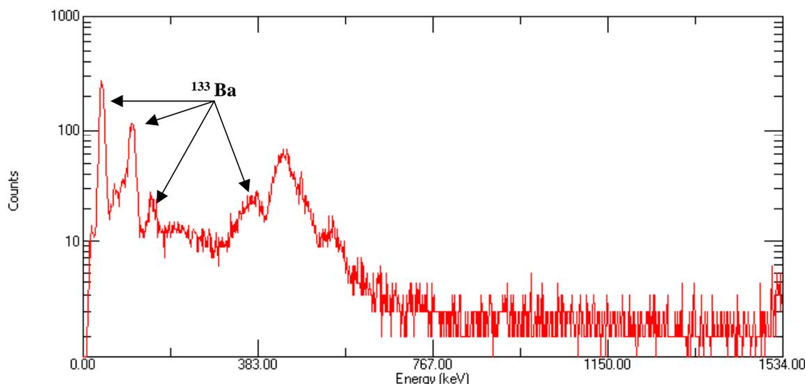
Figure 9 Typical NaI(Tl) spectrum of  $^{133}\text{Ba}$  tracer peaks
