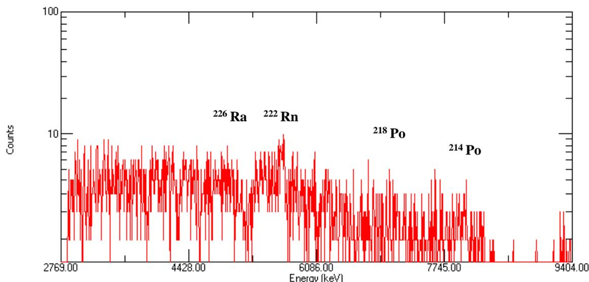
**Figure 8** Very poorly resolved spectrum. Likely Ba contamination.
