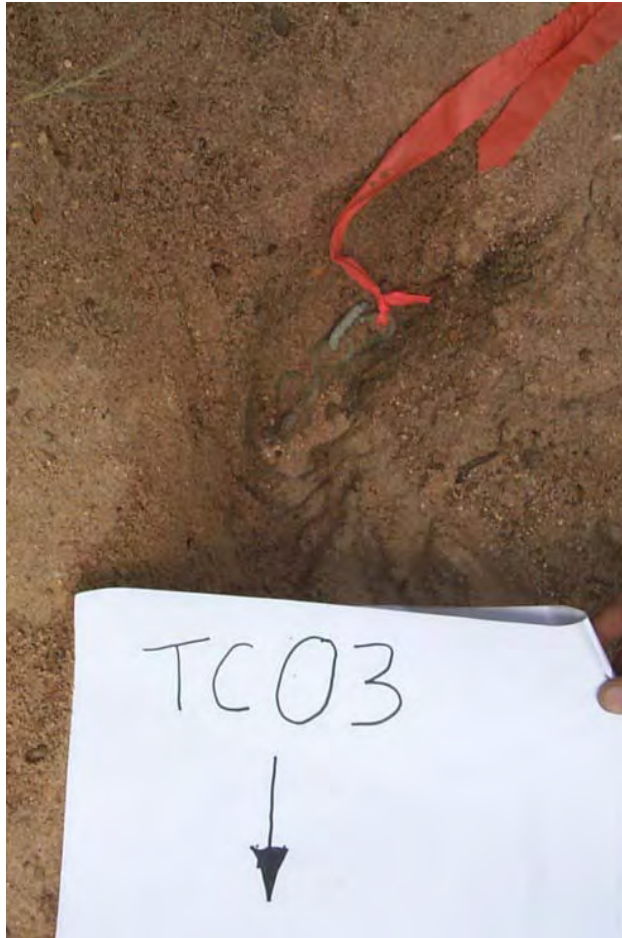
Figure 11 Upstream-directed scour chain at TC03 on 24 October 2000
