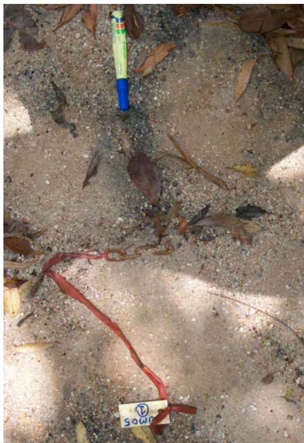
Figure 21 Scour chain UM05-1 (2001) pointing towards the right bank
