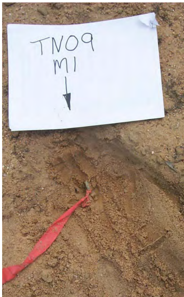
Figure 7 Scour chain at TN09-1 on 24 October 2000 showing that the top link was still orientated vertically and hence had not been scoured during the 1999/2000. Arrow points downstream.
