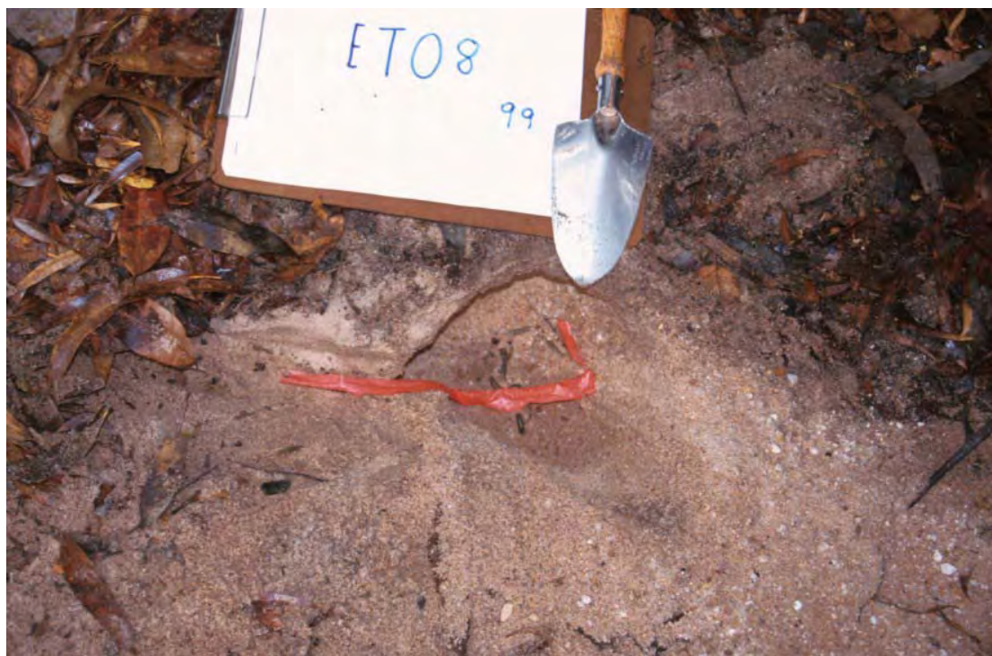
Figure16 Scour chain at ET08 (1999) pointing in an upstream direction. The top link has the flagging tape attached to it.
