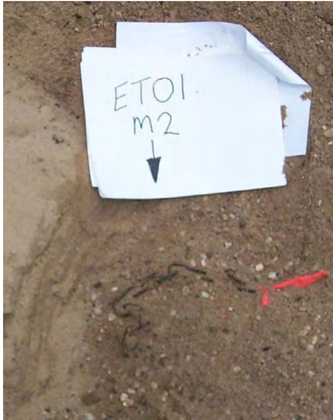
Figure 14 Scour chain at ET01 (2000) directed towards the left bank. Flow direction shown by arrow.
