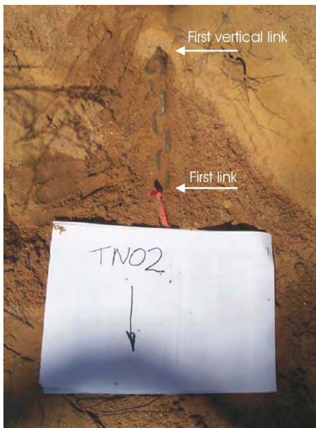
Figure 5 Scour chain at TN02 on 24 October 2000 orientated downstream. Arrow shows flow direction.
