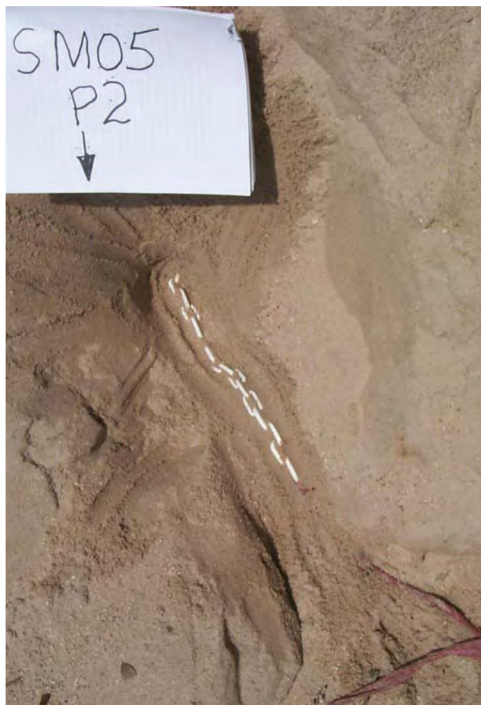
Figure 27 Plastic scour chain at SM05–P2 (2000) pointing almost downstream
