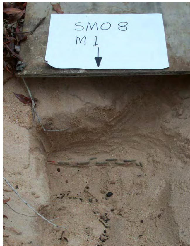
Figure 30 Scour chain SM08-1 (2000) pointing towards the right bank
