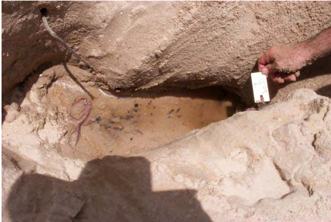
Figure 25 Scour chain SM05-2 had been totally dislodged during the 1998/1999 Wet season and was lying below the water table in November 1999
