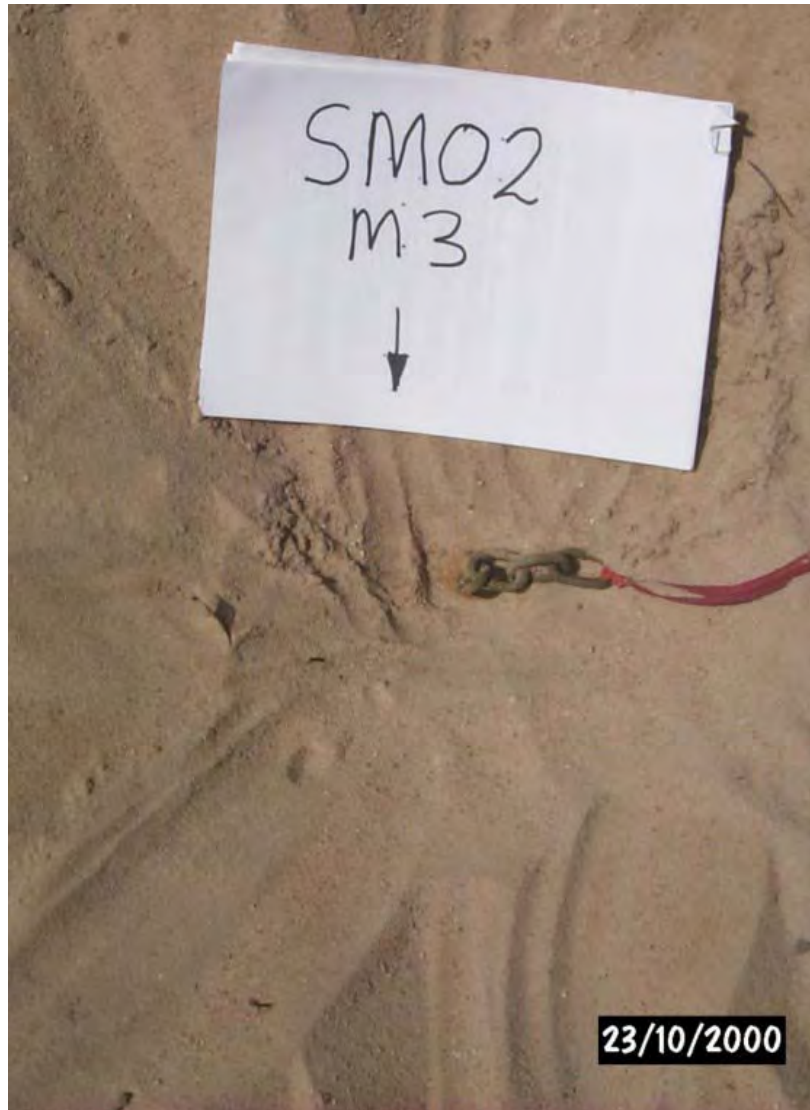
Figure 28 Scour chain SM02–3 (2000) pointing towards the left bank
