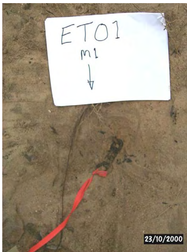
Figure 13 Scour chain pointing essentially downstream at ET01 on 23 October 2000
