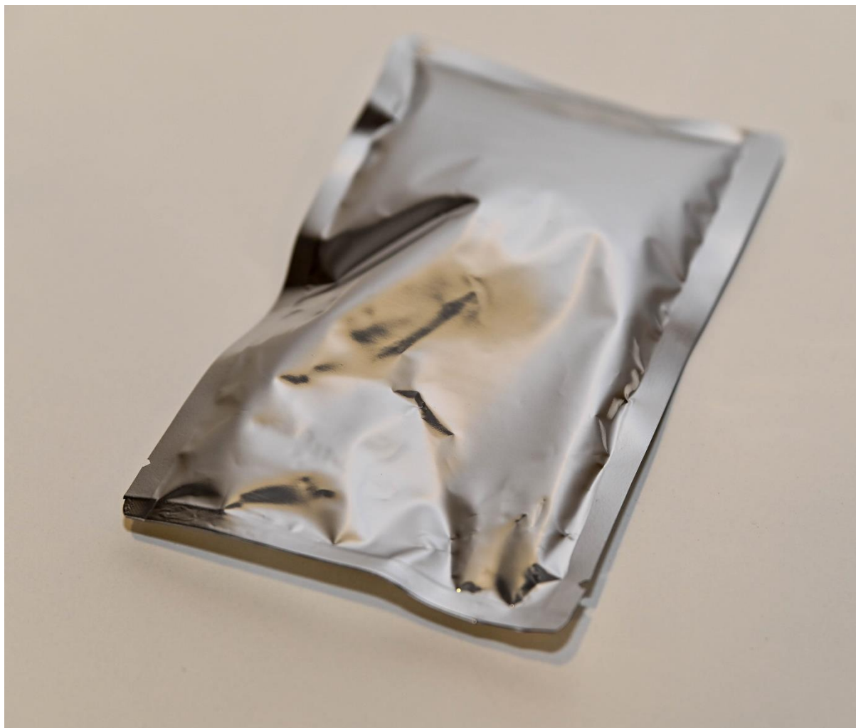
Photo 13 Example of unsuitable foil packaging. Packaging must be opened, slashed or removed to make suitable for treatment.
