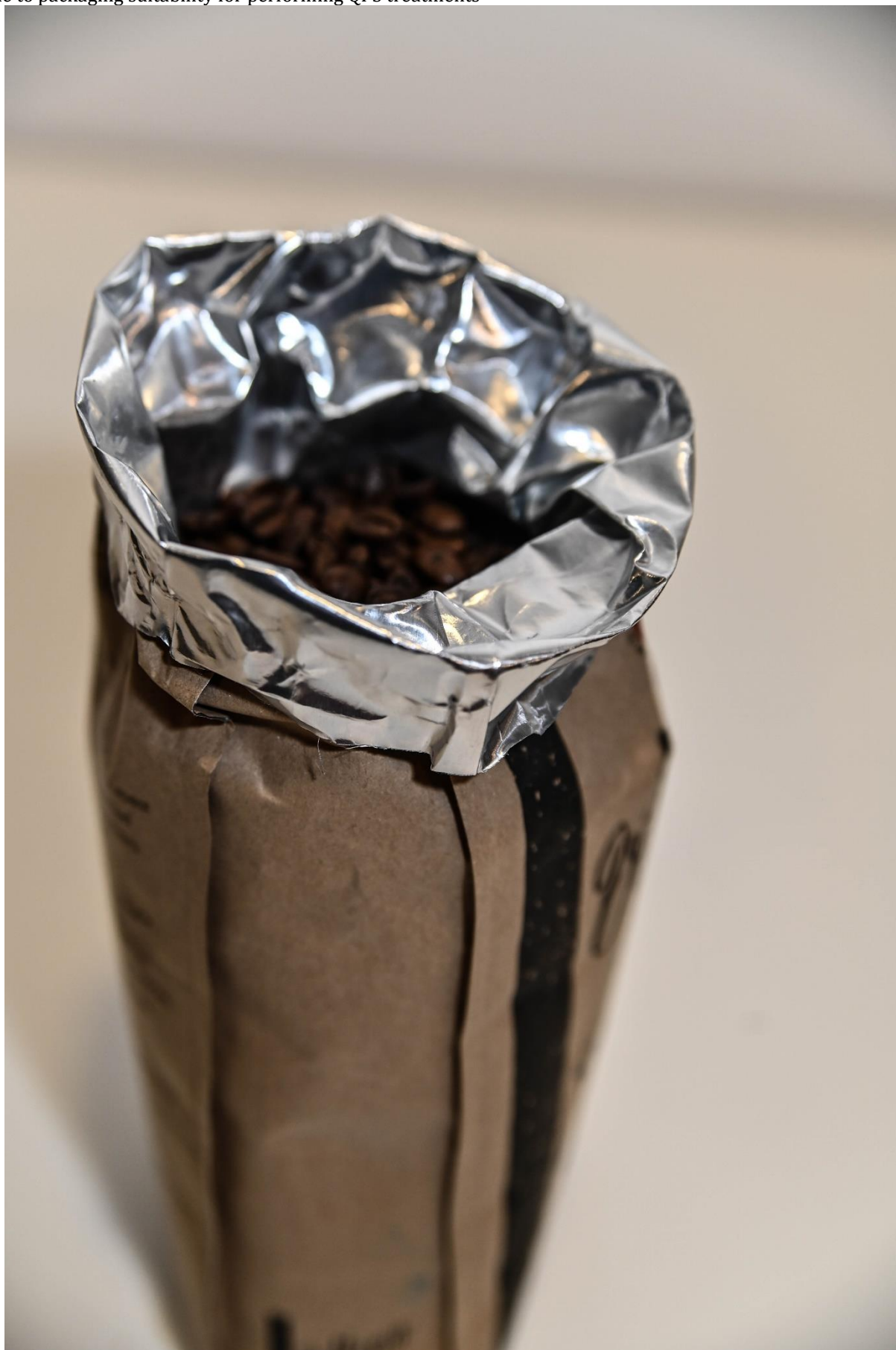
Photo 12 Example of unsuitable paper packaging due to impervious foil liner. Liner must be opened, slashed or removed to make suitable for treatment.
