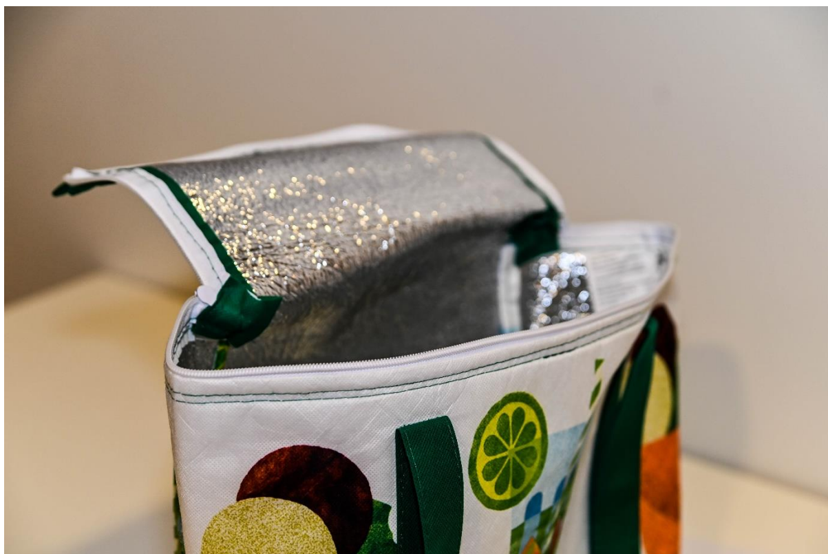
Photo 8 Example of unsuitable cloth packaging due to impervious foil liner. Liner must be opened (as presented above), slashed or removed to make suitable for fumigation.
