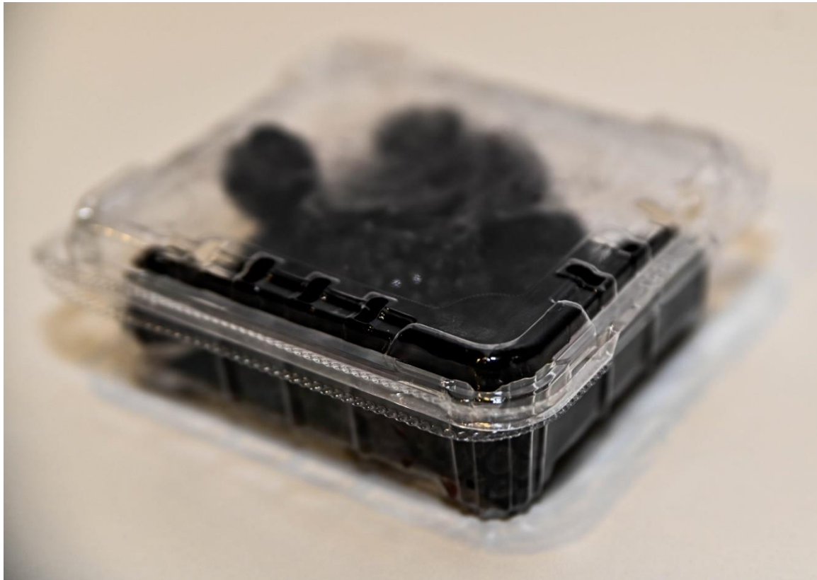
Photo 1 Example of suitable plastic packaging. Otherwise impervious wrapping, perforated with four or more holes, with a diameter larger than 6mm, for every 100mm x 100mm of surface area. Positioning of the holes allows for stacking without blocking.
