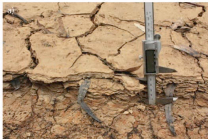
Figure 3-1. Sediment drapes (deposition) were more common during slow rates of recession and can encourage vegetation establishment.
