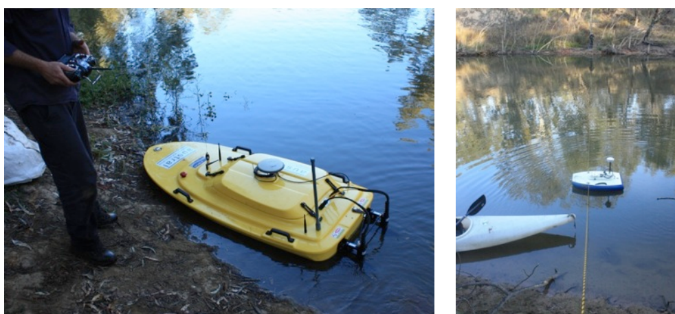
Figure B-1. Instruments used to collect field data for development and verification of the hydraulic model: (left) Sonar bathymetric survey boat, (right) Acoustic Doppler Current Profiler (tethered to a rope to obtain velocities across fixed cross sections).
