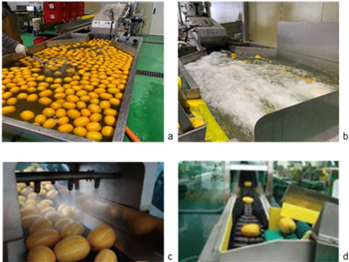
a: First washing step with immersion bath. b: Second washing step with high-speed water jets in dump tank. c: Alternative second washing step with high-pressure water spray on conveyor belt. d: Hot air drying and movement to grading via conveyor belt. Source: APQA (2021)
