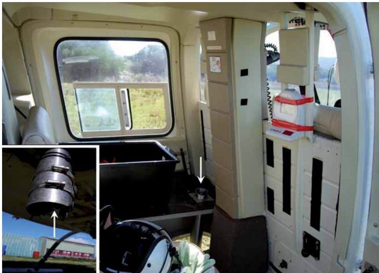
Figure 12. Arrangement of baits, drop tube and stopwatch inside helicopter. Inset shows microswitch for automatic logging of dropped bait.
