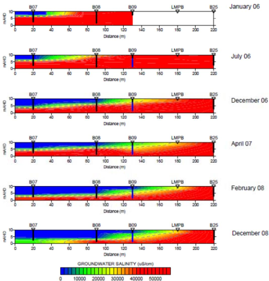
Figure 18. Transect 3 sonde profile data indicating freshwater lens development resulting from Living Murray pumping.
