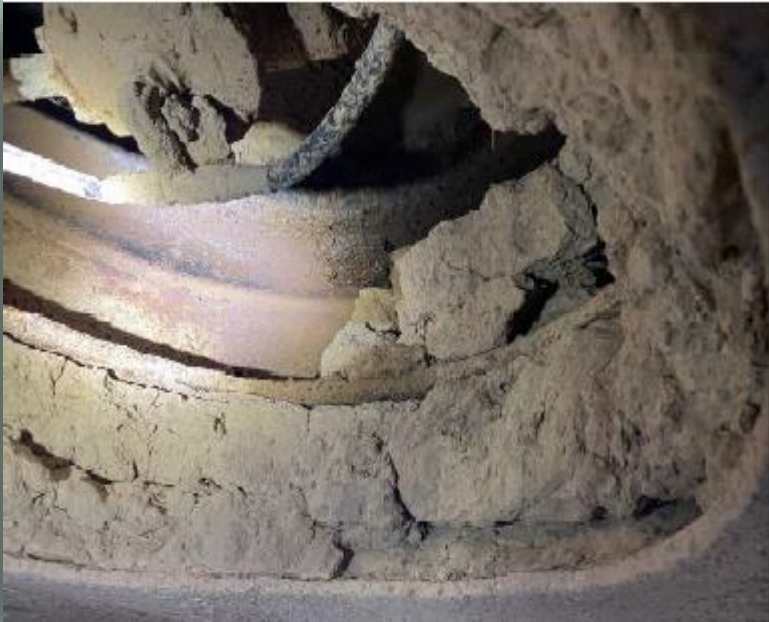
Excavator turret – no attempt at cleaning
