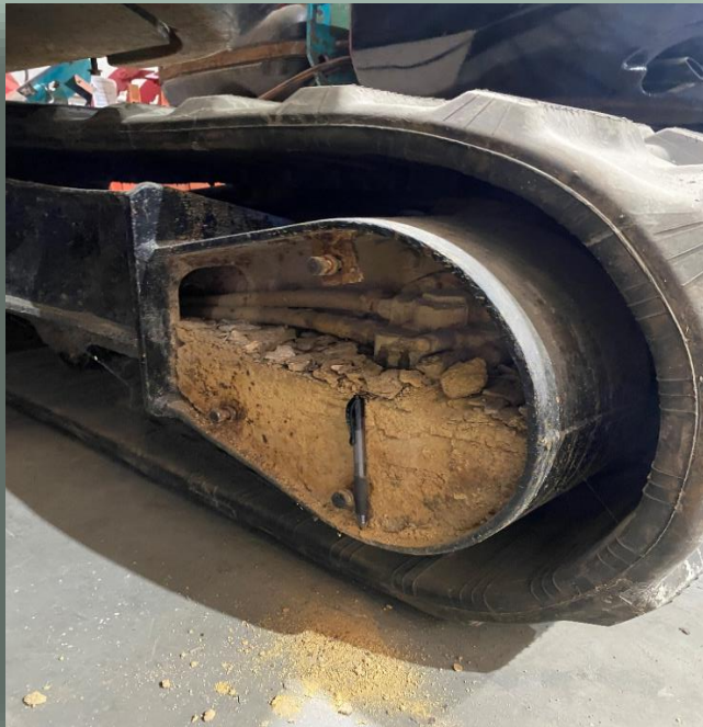
No removal of drive motor panel or attempt to clean.
