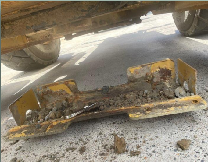
Belly plate not removed and no attempt to clean
