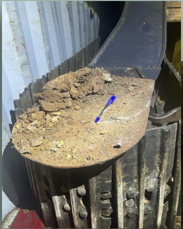
Excavator drive arm – full of soil & prohibited packing – no attempt at cleaning
