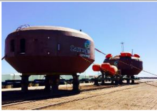
CETO Unit 2 prepared for deployment quayside along CETO Unit 3 (L), Carnegie operations team member controlling position of Buoyant Actuator from deployment barge (R)
