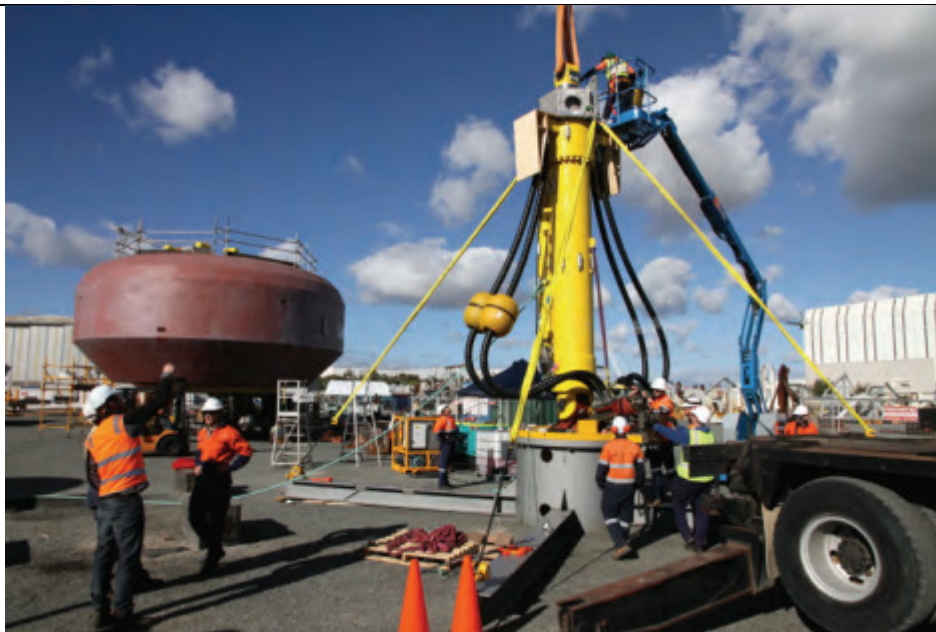
Pump integration testing at BAE Systems, Henderson
