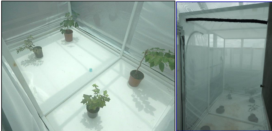
Figure 18 – Examples of choice oviposition trials conducted in the 215 x 140 x 210 cm cage.
