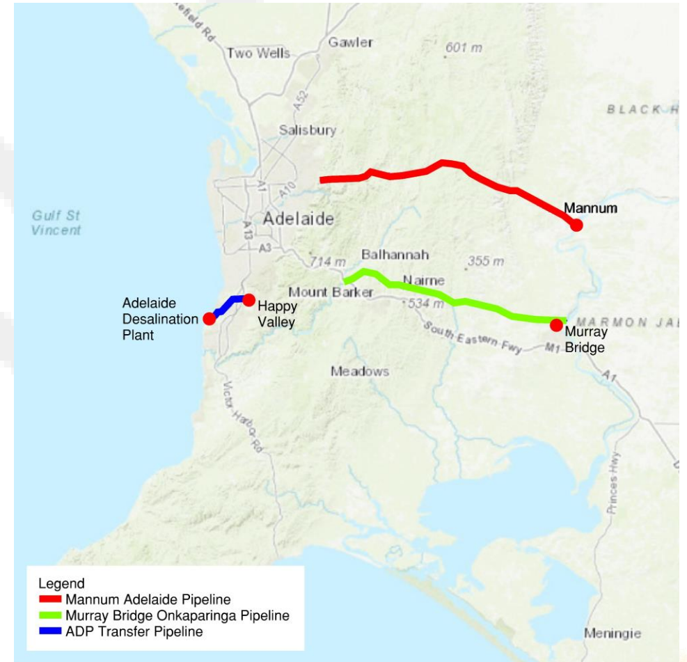
Figure 3: SA Water Metropolitan Network – Major Pipelines
