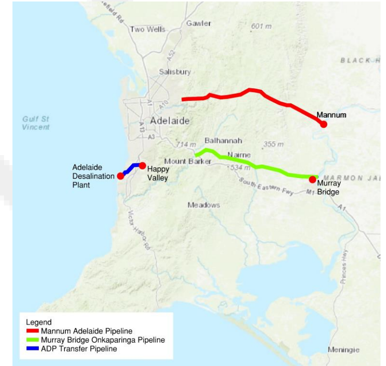
Figure 1: SA Water Metropolitan Network – Major Pipelines
