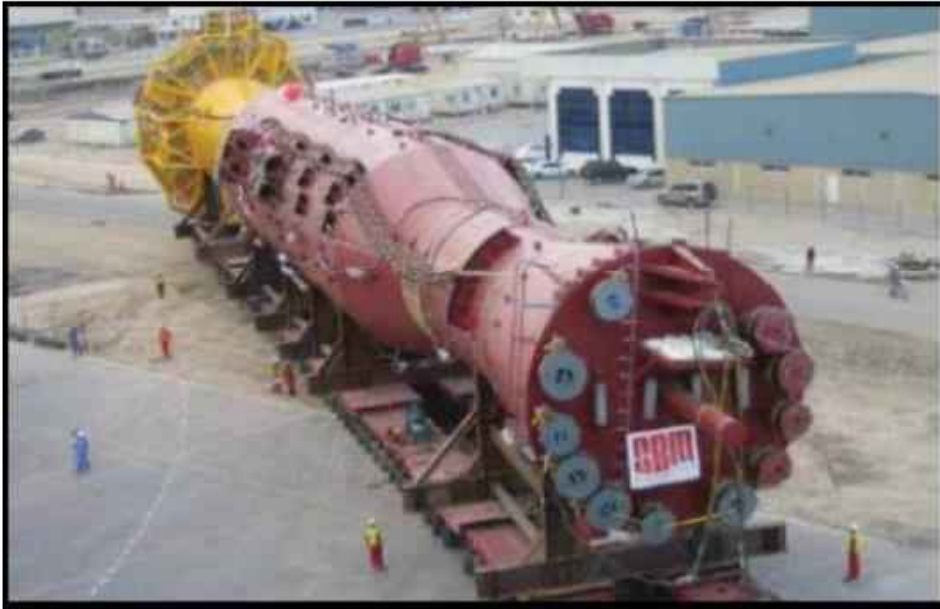
Figure B-1: Riser Turret Mooring (RTM).
