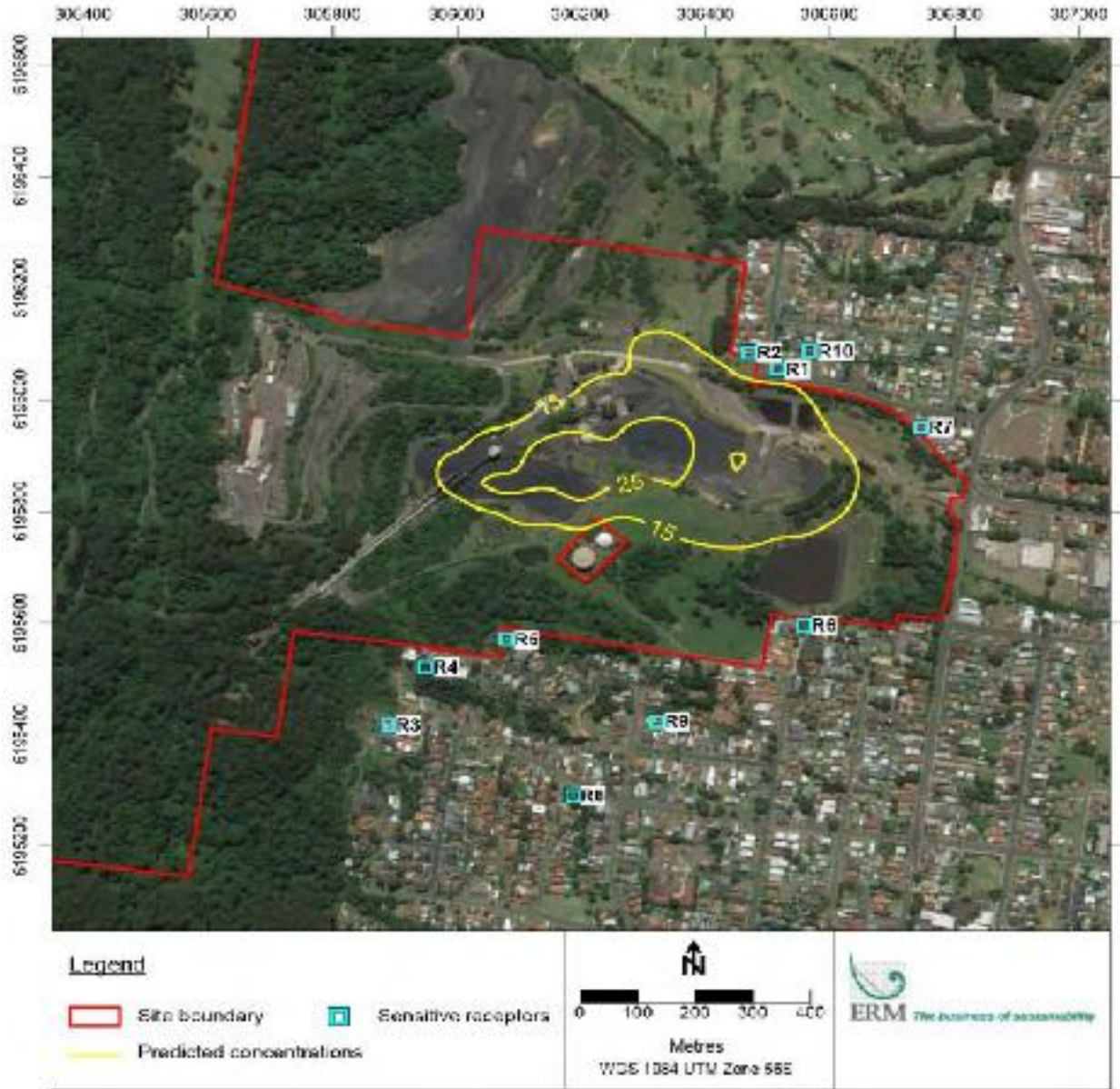
Figure 9 – Predicted annual average cumulative PM 10 concentrations due to the proposed operations and background concentrations (Scenario 2).
