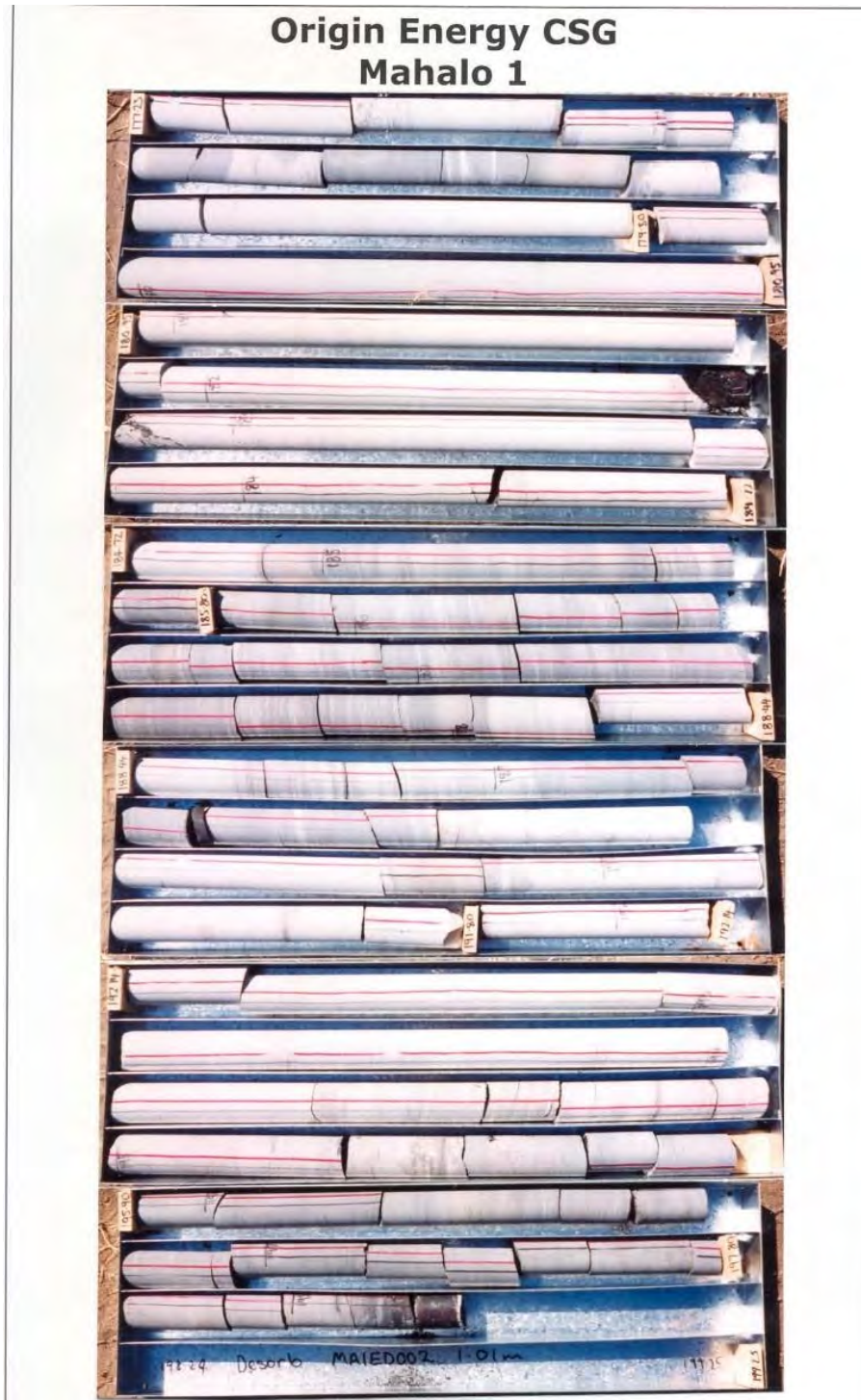
Photo 2-3 Core Photos from MAH1 – Rewan Group from 177.23 mbGL to 197.46 mbGL
