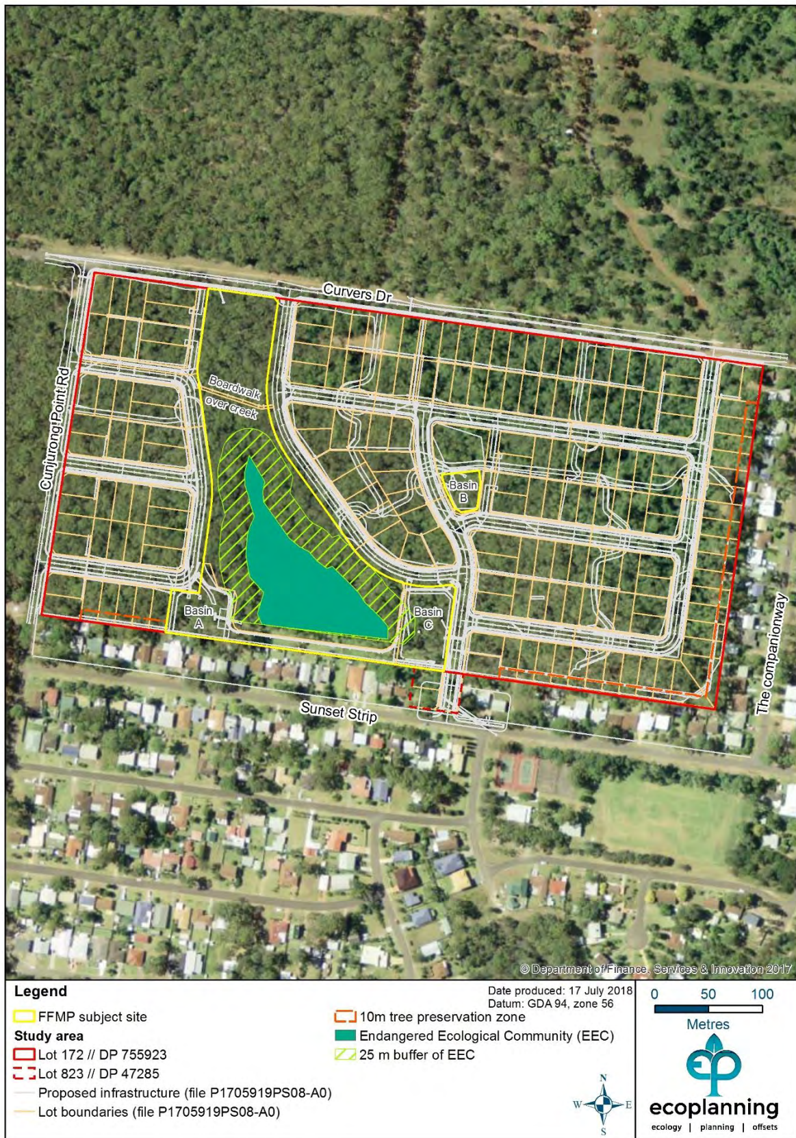
Figure 1.2: EEC area, 25 m buffer, Bushland Reserve, basins and the proposed development.
