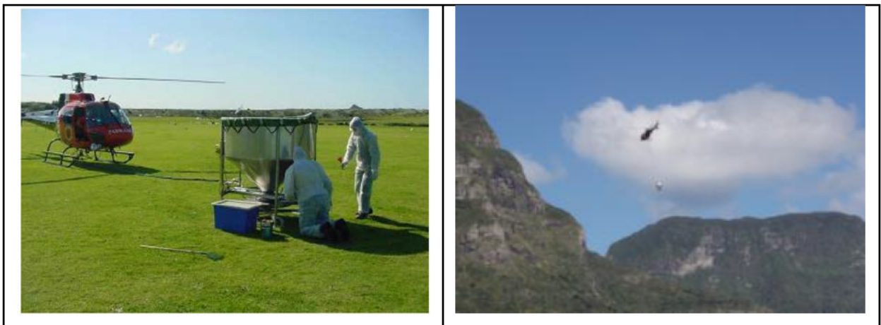
Figure 15 Custom built spreader bucket being prepared and in use on LHI during 2007 trials.
