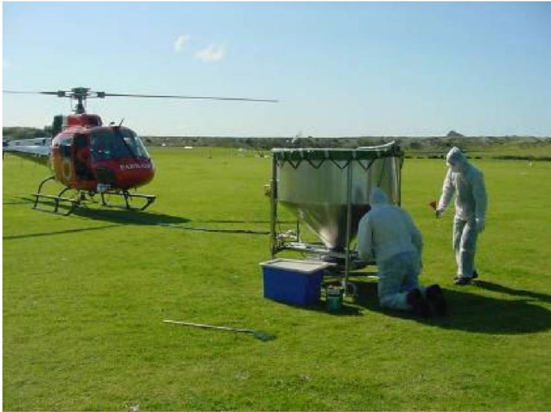
Figure 2: Custom built spreader bucket being prepared on LHI.
