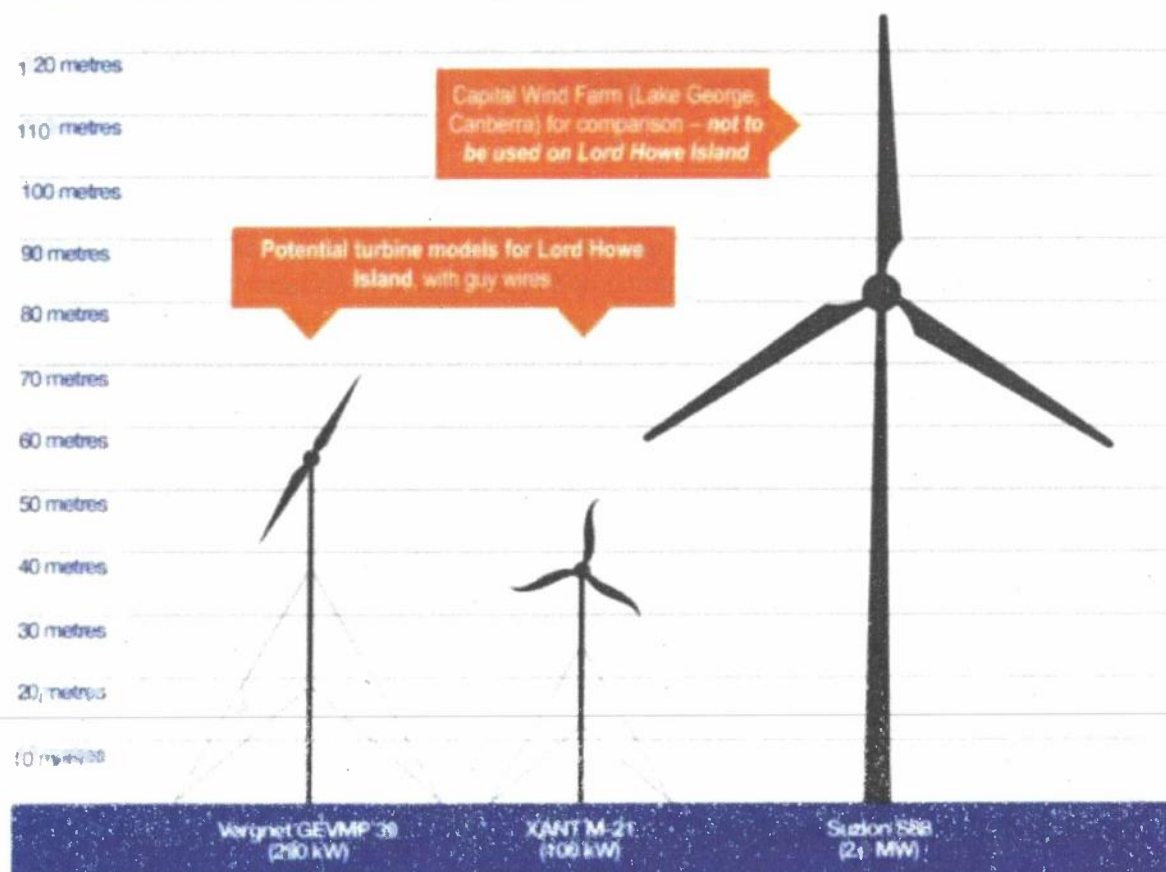
Figure 1: Height and rigging comparison between the Vergnet the XANT and the Suzlon 80 turbine (installed at the Capital Wind Farm, Lake George, NSW).
