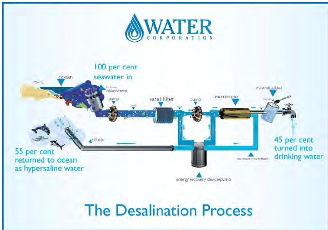
Figure 1-4 Desalination process diagram
