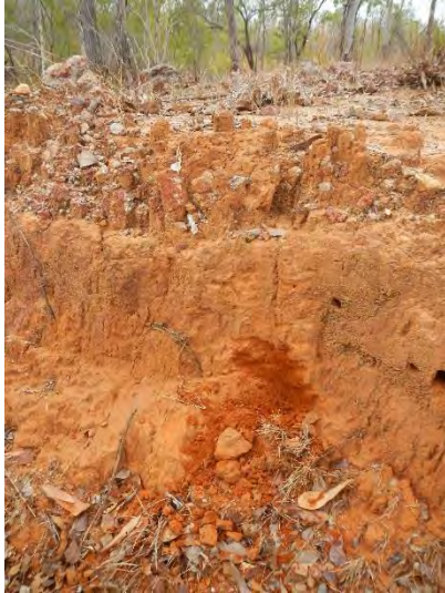
Figure 7 An exposed Kandosol soil profile at a road cut near Area 1 on Kingvale Station. Note the potential for soil piping (sub-surface drainage through macropores) at depth as indicated by dark areas in centre right of picture, as well as stony fragments.
