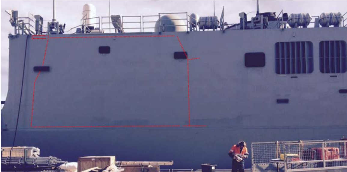
Photo 1: This photo of a similar vessel to the Ex-HMAS Adelaide demonstrates the location of the section of the starboard hanger structure that has separated from the vessel. It is marked in red.
