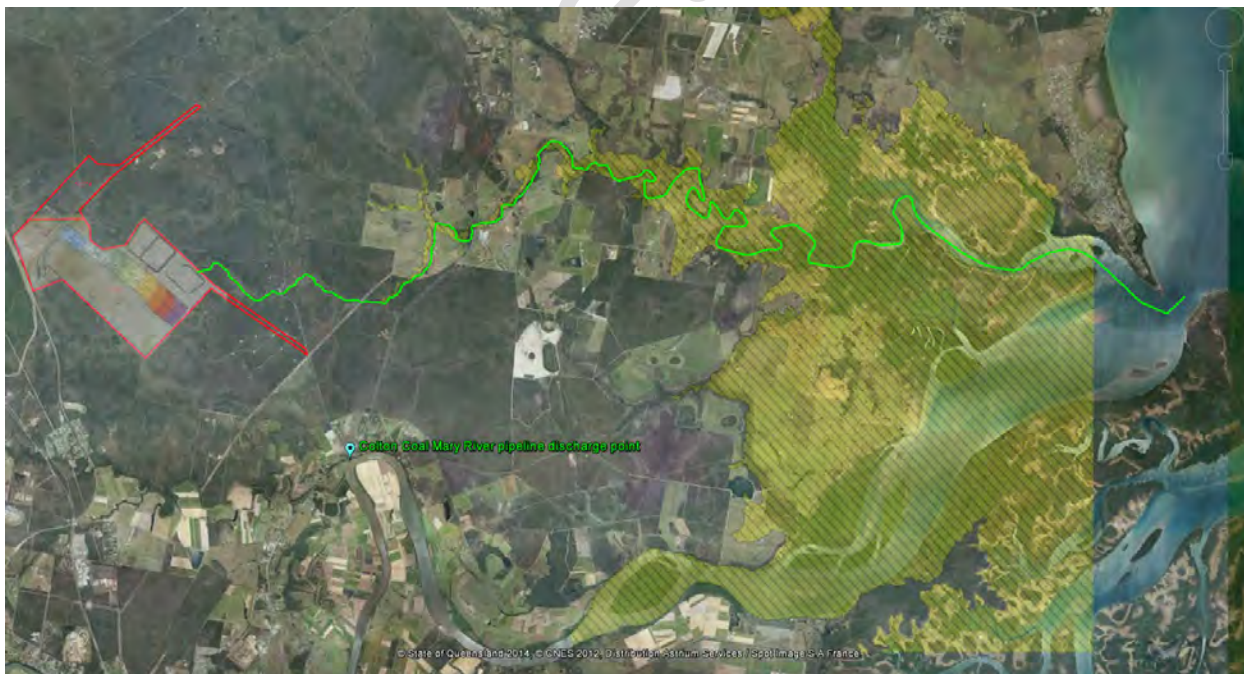
Figure 28 – Catchment downstream of Colton Coal mine site showing HEV zones (yellow hatched area), the proposed controlled release point into the Mary River (blue icon) and the path that an uncontrolled release from the site would take after discharging from the main dam
