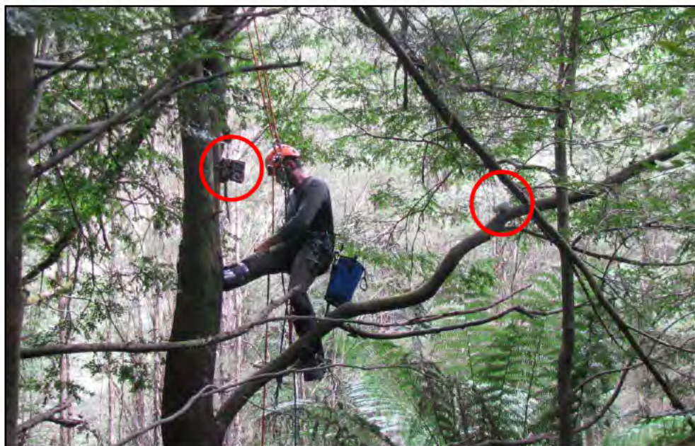
Figure 1. Tree canopy specialist setting a camera trap consisting of a Reconyx survey camera (circled left) set 2–3 m from a bait holder containing creamed honey (circled right).
