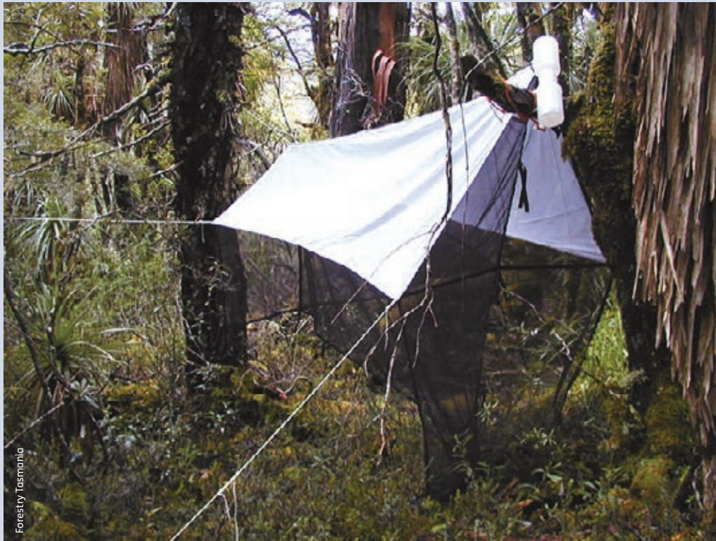
Figure 1.31: Malaise trap for sampling flighted arthropods, installed in the 600-metre altitude plot at Warra
